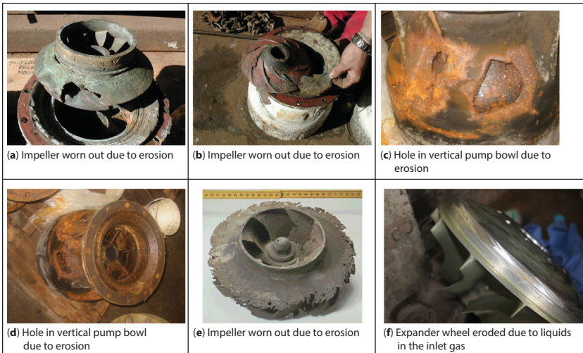
Figure 3.2 Examples of erosive wear failures.
