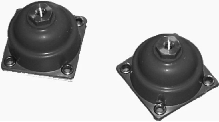
FIGURE 39.11 Fluid-elastomer mounts are moderately well damped and exhibit stiffening characteristics similar to cup mounts but have limited load ratings and are not fail-safe except within captured metal housings. They comprise silicone gel-filled elastomer body and axial spring to support vertical load.
