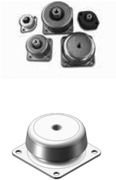
FIGURE 39.10 Housed cup mount—fail-safe design, captured molded elastomer element, mildly increasing stiffness in the principal directions, relative deflection capability less than 0.5 in., various types.
