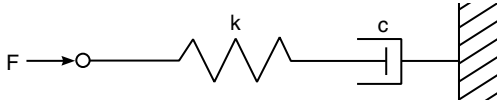
FIGURE 9.3 Schematic representation of a series combination of a spring and a damper.
